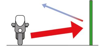
Noistop acoustic wall: Shielding and absorption
