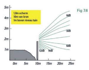
For high locations of the sound source with respect to screen and receiver
