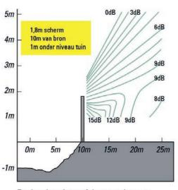
For low locations of the sound source with respect to screen and receiver
