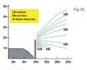
For high locations of the sound source with respect to screen and receiver
