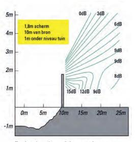
For high locations of the sound source with respect to screen and receiver
